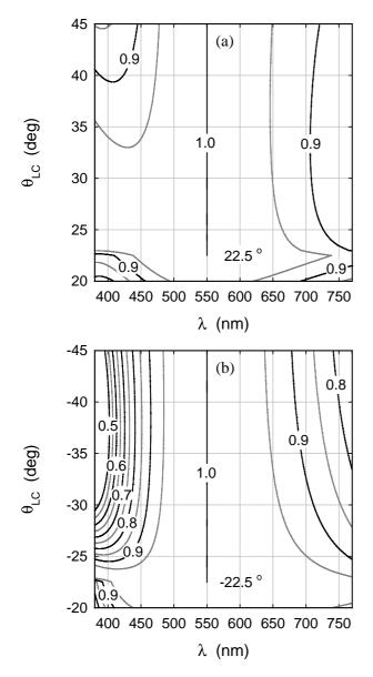
Fig. 4. Iso-reflectance curves for the two in-plane optical geometries as a function of the wavelength ( $\lambda$ ). The calculations were performed along the maximum reflectance line obtained with fixed wavelength of 550 nm.
