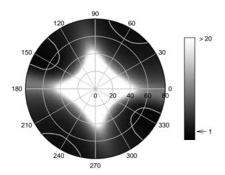
Fig. 5. Gray scale representation of the iso-contrast map for a reflective LCD cell with  $\theta_{LC} = -22.5^{\circ}$ . The white solid curves represent the inversion lines of contrast.
