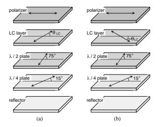
Fig. 1. Two in-plane optical geometries of a reflective LCD: (a) the counter-clockwise rotation and (b) the clockwise rotation of the average optic axis of the LC layer. A combination of the HW and QW plates is used for the WQ plate.
