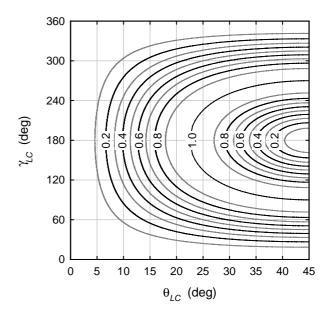
Fig. 3. Iso-reflectance curves given in the plane of the molecular rotation or the rotation of the average optical axis ( $\theta_{LC}$ ) and the phase retardation ( $\gamma_{LC}$ ) of the LC layer for normal incidence.
